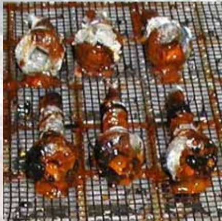
Competitor's extended life coating in ACQ wood after 1248 hours SST
