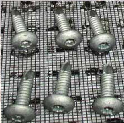
Fastec FX2™ in ACQ wood after 1248 hours SST
